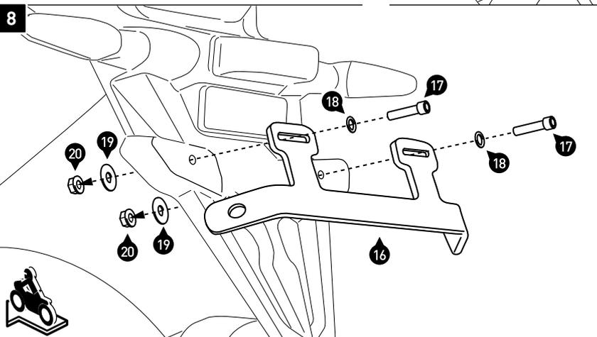
Connect both side carries (10) and (11) to the mounting brackets (1), and (6) by using the fasteners (21), as shown in the detail drawing. Now connect the crossbar (16) to the side carriers by using the fasteners (21).
