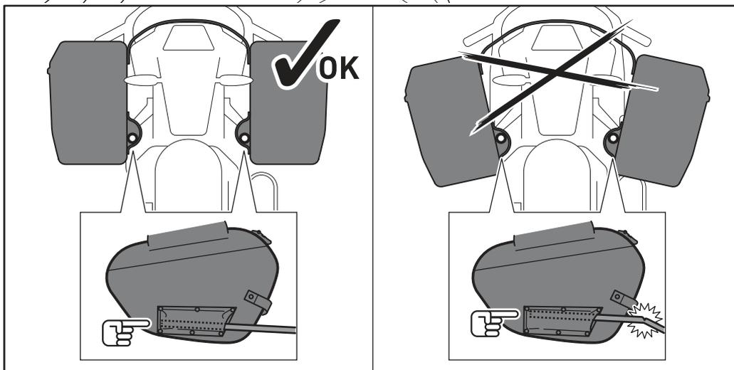
Fasten the panniers (3) with the Velcro flaps over the rear (passenger seat) of the motorcycle, as shown in the drawing.
